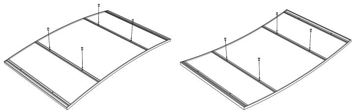
Ceiling rafts are delivered in one piece making them quick and easy to install. Flexible design and adjustable to various heights using steel cables.
