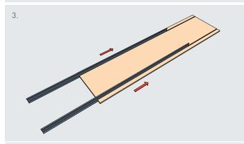
Push the T-profiles into the grooves on the reverse side of the Corridor. Centre the profiles. Tile overhang 25mm right and left.
