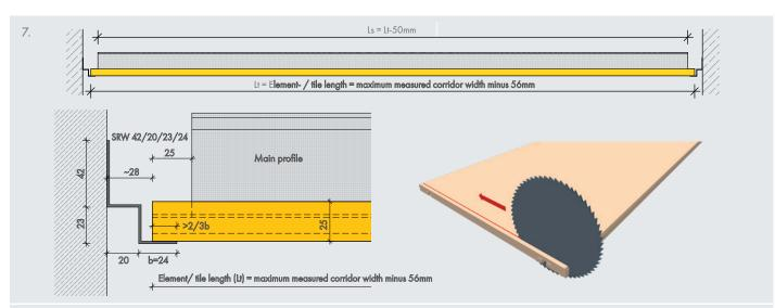
The HERADESIGN® Corridor is available to order in every required length up to a maximum tile length (Lt) of 2400mm. To allow for structural tolerances, the main profiles are 25mm shorter than the tile, at both ends. The elements can be shortened by up to 50mm when required. This can be carried out with a hand saw, circular saw or with a table saw.
