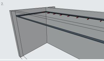
Install the perimeter angle using approved plugs and screws. Maximum spacing of the fixings 400mm. The perimeter angle should be mitred at the corners.
