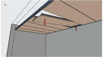
The Corridor are demountable by gently lifting the tile up and moving to the side.
